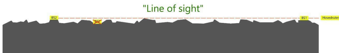
Figure 4: Tunnel wall seen from above. No obstacles between BS units — “Line of sight”
